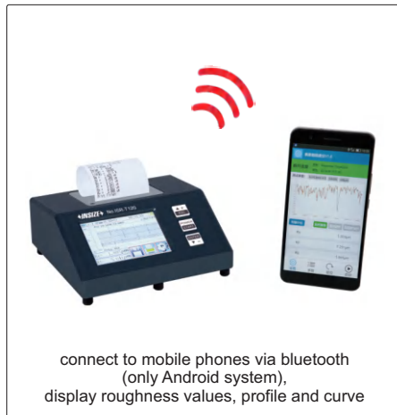
operate roughness tester by mobile phones
