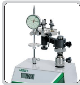
check the measuring force of dial indicators
