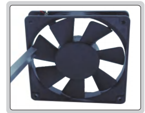
measuring blade to sidewall gap
