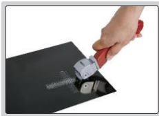
step 1: make grid cutting on surface
