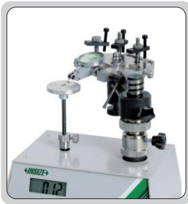
check the measuring force of dial test indicators
