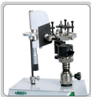
check the measuring force of indicating micrometers
