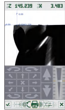
check cutting edge wear
