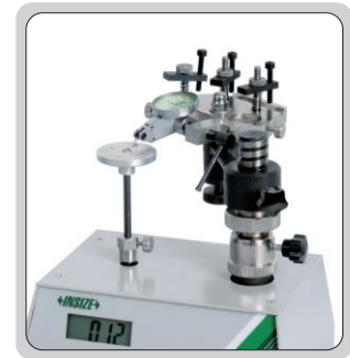
check the measuring force of dial test indicators
