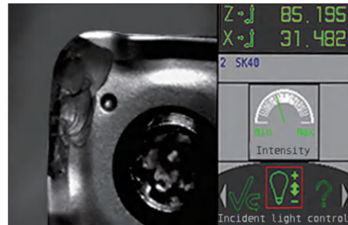
check cutting edge wear
