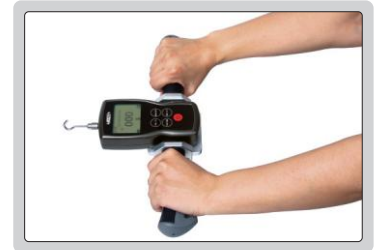
pull test with two handles
