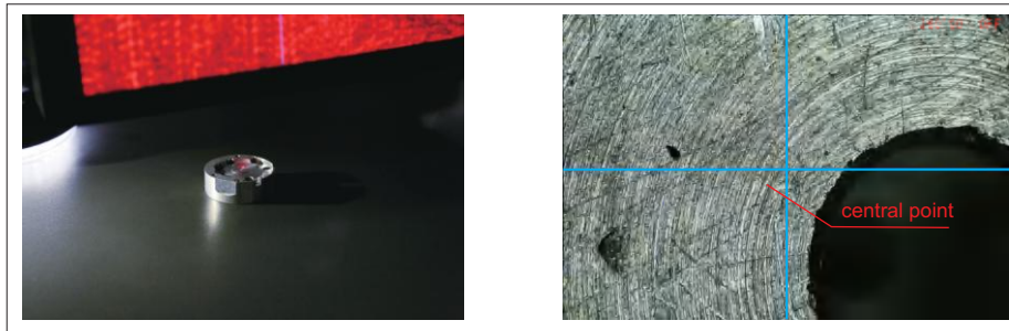
laser indicator locates the central point
