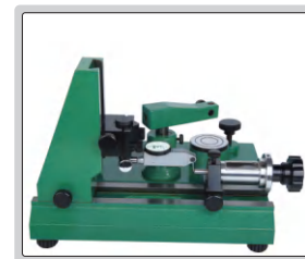
inspect accuracy of test indicators
