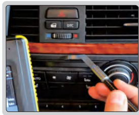
measuring gaps on the car dashboard
