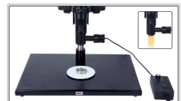
for smooth surfaces and small holes, brightness is adjustable
